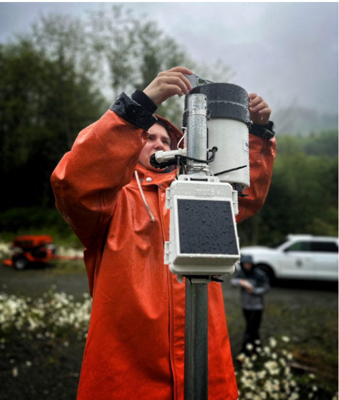
A Prince of Wales Alaska Youth Stewards crew member adjusts tipping bucket and rain gauge on Port Saint Nicholas Road. This device measures rainfall. Photo: Zofia Danielson
